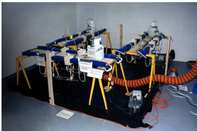
Fig. 7. Apparatus used to test beam pairs under load in various aqueous environments. Six sets of beam pairs were enclosed in flexible hose and weights were hung from the beams to load beam pairs in a four point bending configuration. Aqueous solutions were circulated through the flexible hose with peristaltic pumps.
